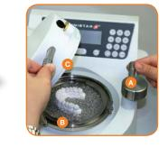
After cooling time has elapsed, open pressure chamber: A open locking handle
