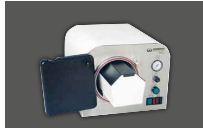
DEG-2 with polymerisation trough, available as accessory
