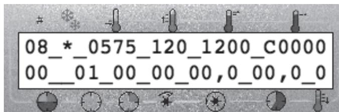
7. Press the → key. The cursor will jump to the next field, **Pre-heating time**. Enter the desired value via the keypad or the + and – keys.
