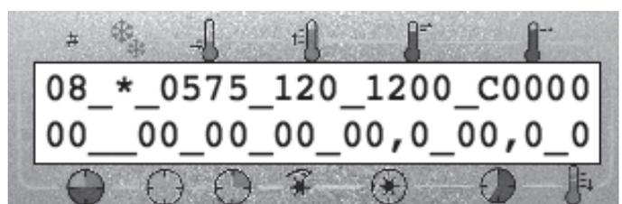
6. Press the → key. The cursor will jump to the next field, **Drying time**. Enter the desired value via the keypad or the + and – keys.
