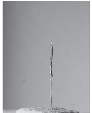
If the surface of the silver wire does **not show any signs of melting**, the temperature is **too low**.
