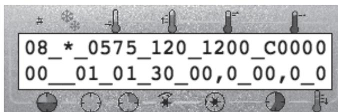
9. Press the → key. The cursor will jump to the next field, **Vacuum time**. Enter the desired value via the keypad or the + and – keys.
