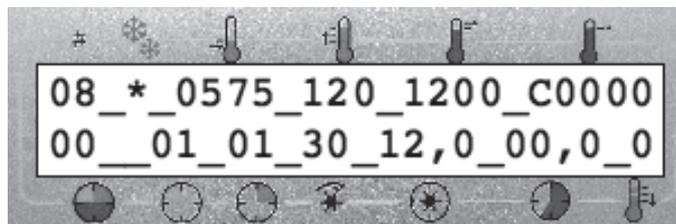
10. Press the → key. The cursor will jump to the next field, **Firing time**. Enter the desired value via the keypad or the + and – keys.
