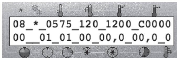
8. Press the → key. The cursor will jump to the next field, **Vacuum**. Enter the desired value via the keypad or the + and – keys.
