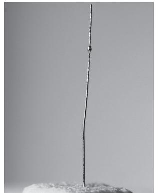
If the **silver wire** has partially or completely melted to a clump, this means that the temperature is **too high**.
