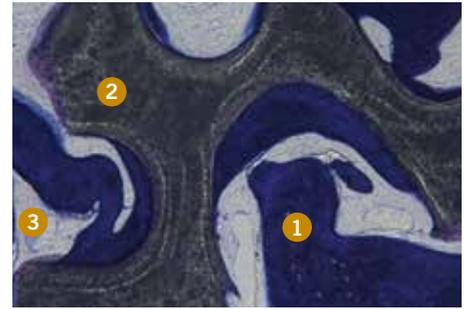
Interconnecting 3D pore system and a large interior surface
